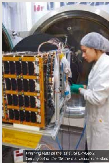
Finishing tests on the satellite UPMSat-2. Coming out of the IDR thermal vacuum chamber.
